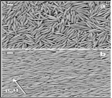
This alignment more efficiently couples the magnetic field from magnetized particles into the head structure. Tape is simpler to orient, since it travels in a linear direction, so magnets placed above the wet coated tape prior to oven curing of the coating binder will provide a particle-oriented media.
