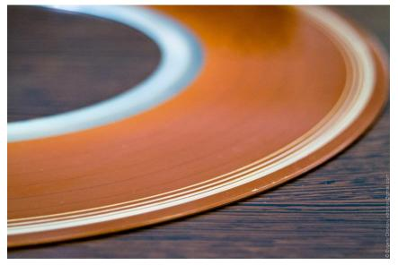
**Ski-Jump** – refers to an edge condition caused by rotating polishing pads which dish out the central part of the disk leaving a slightly raised outer edge. The edges of a recording head flying over this curvature could mechanically interfere with the disk causing a "head crash"
