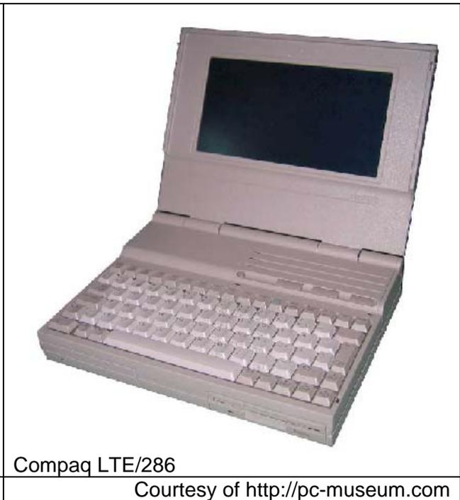
Only one year later, the re-packaged \$5,000 6.7 pound 2" thick LTE/286 with a 2.5" 40MB drive joined the notebook market. The claimed 4.8V 5.0 A/h battery life of up to 3.5 hours was a gross exaggeration, the real life was much shorter. The biggest power hogs were the display screen and drive, and users could not stray far from wallpower.
