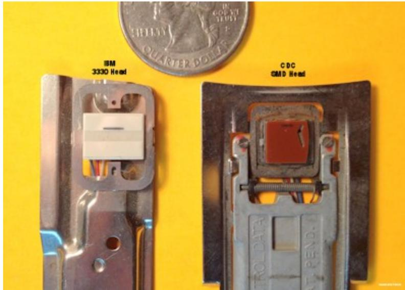
Figure 3 –IBM 3330 head (left) and CDC SMD head (right)
