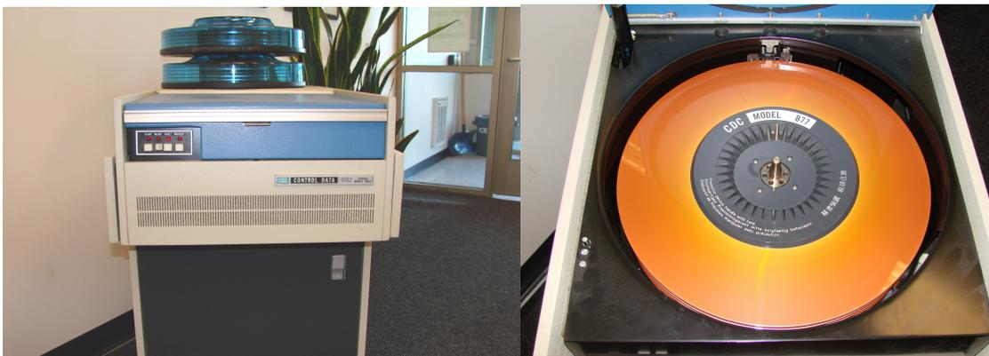
Figure 2 - CDC 9762 SMD and two packs    CDC 877 80-MB Pack mounted in drive
