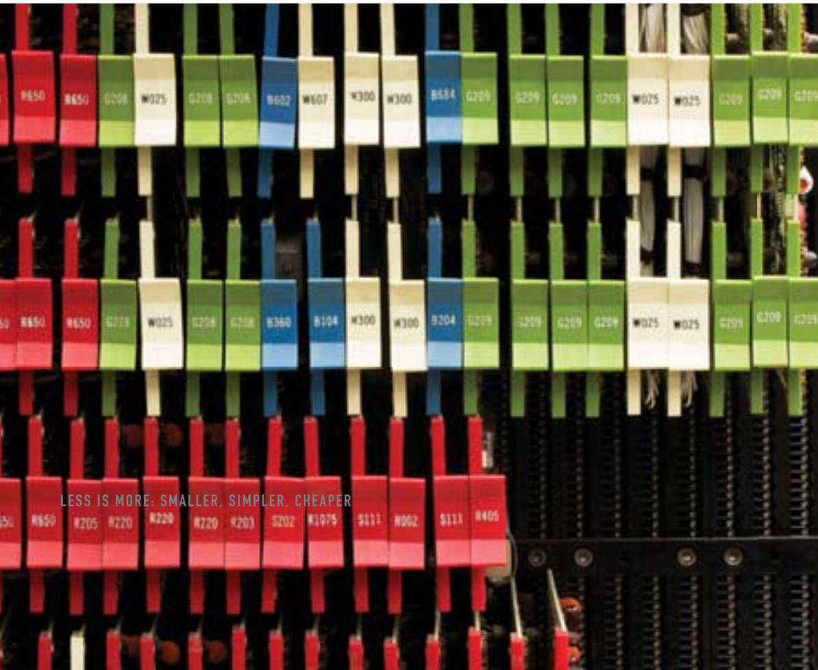
Close-up of DEC PDP-8 flip-chip modules
