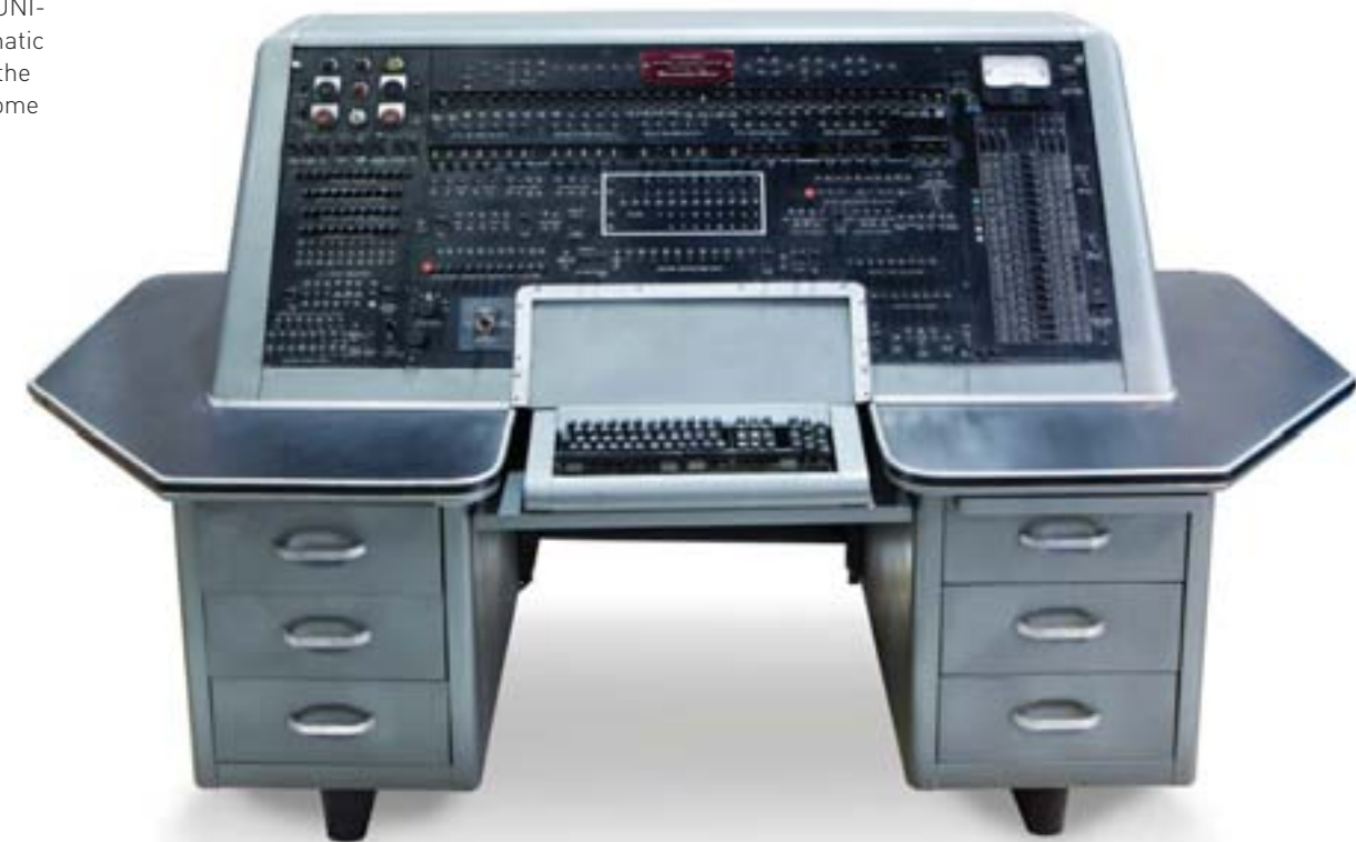
UNIVAC I Supervisory Control Console, Remington Rand, US, 1951
