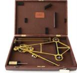
The Integrator quickly calculates the bending properties of any railroad rail design placed under it. The user need only trace the outline. This complex mechanism calculates static and inertial moments as a drawing is traced.
