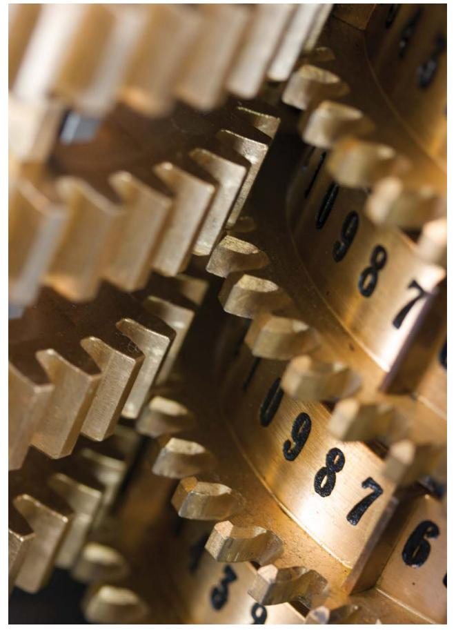
Figure wheels engaged with adjacent sector wheels during addition.
