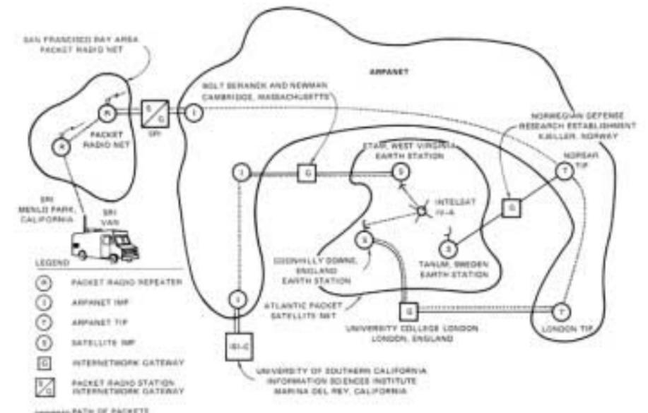
FIGURE 1 FIRST ARPA MULTINETWORK DEMONSTRATION
