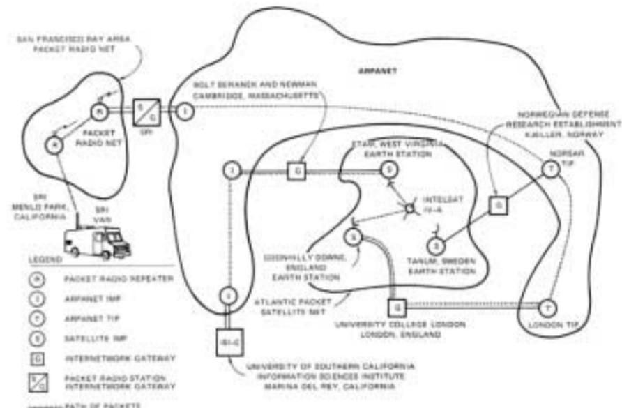
FIGURE 1 FIRST ARPA MULTINETWORK DEMONSTRATION
