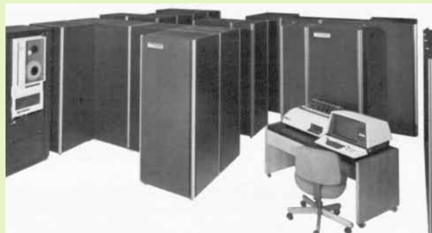
The Denelcor HEP was a uniform shared memory multiprocessor that used fine-grain multithreading to tolerate memory latency, synchronization latency, and even functional unit latency. Six systems were delivered to customers during the years 1981-1985.
