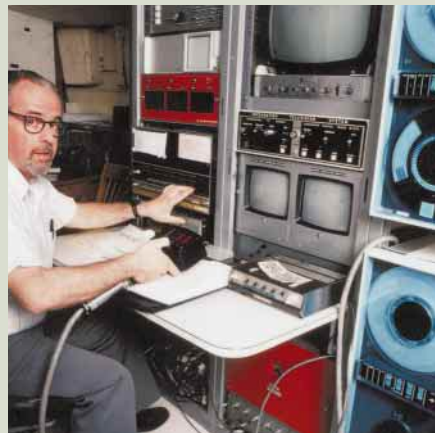
The NOVA mounted in a telescope control system and in use, circa 1981, at the University of Texas (the operator rests his hand on NOVA control panel)
