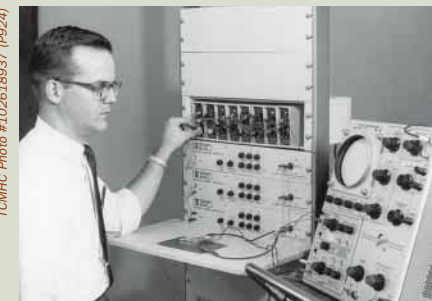
DEC's beginnings lay in producing small logic modules like this engineer is adjusting here.
