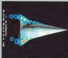
National Aerospaceplane model showing density contours in cross-flow planes.
