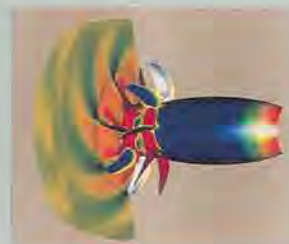
Calculated pressure field radiated by an unducted fan engine. Computer modeling is being used to accelerate the design of more powerful and efficient aircraft propulsion systems. (Courtesy John J. Adamczyk, NASA Lewis Research Center)
