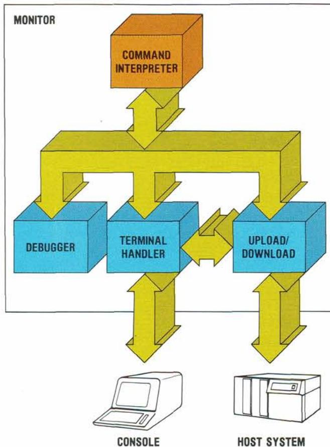
Fig. 1. Monitor Block Diagram
