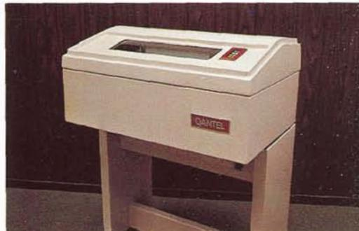
Model 5041 Line Printer prints at rates up to 300 lines per minute and is also fully buffered. One additional line printer can be connected to Systems 1100 and 1200.
