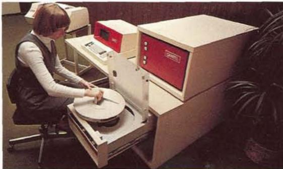
QANTEL Model 3001 Disc Drive provides six million characters of data storage: three million removable for off-line storage, and three million for fixed information. Model 3101 provides 12 million characters of data storage, six million fixed and six million removable.
