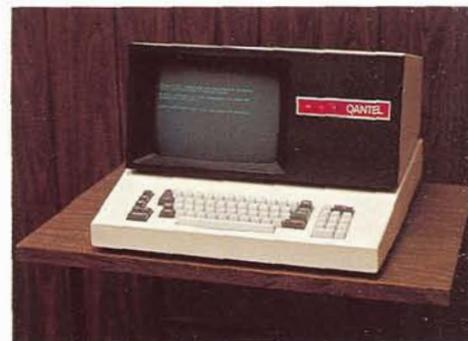
QANTEL's Model 4011 Video Terminal has all the features of the 4001 Video Terminal plus a large, 1728-character screen. The Video Terminals all have the capability of communicating with the computer via telephone lines.
