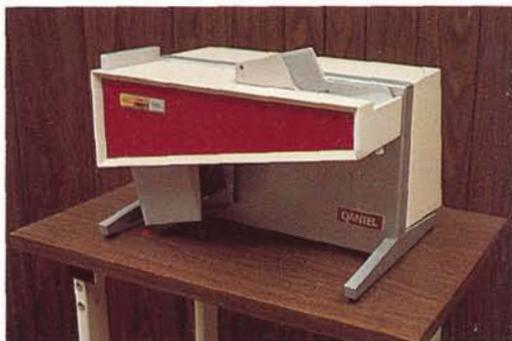
QANTEL Model 5301 Card Reader reads standard 80-column punched cards at a rate of up to 500 cards per minute, for users who already have a card-based system of data storage.
