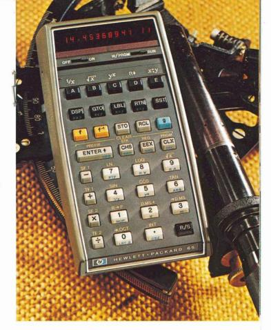
To use a pre-recorded program, you simply insert the appropriate card into the lower slot on the right side of the calculator. The instructions on the card will be automatically transferred to the HP-65's program memory in just 2 seconds.
