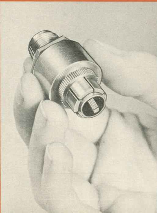
When installed in ERA Magnetic Storage Drums this widely used ERA Magnetic reading-recording head is positioned 0.002" from the drum surface—and maintains this setting during all normal conditions of shipment or use. Low impedance coils permit locating the drum remotely from associated electronic equipment.
