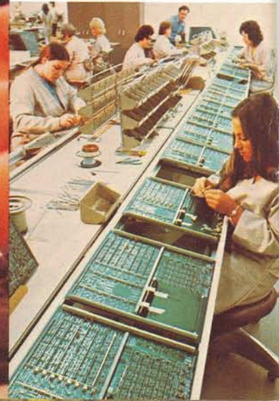
Pretested components being assembled and inspected.
