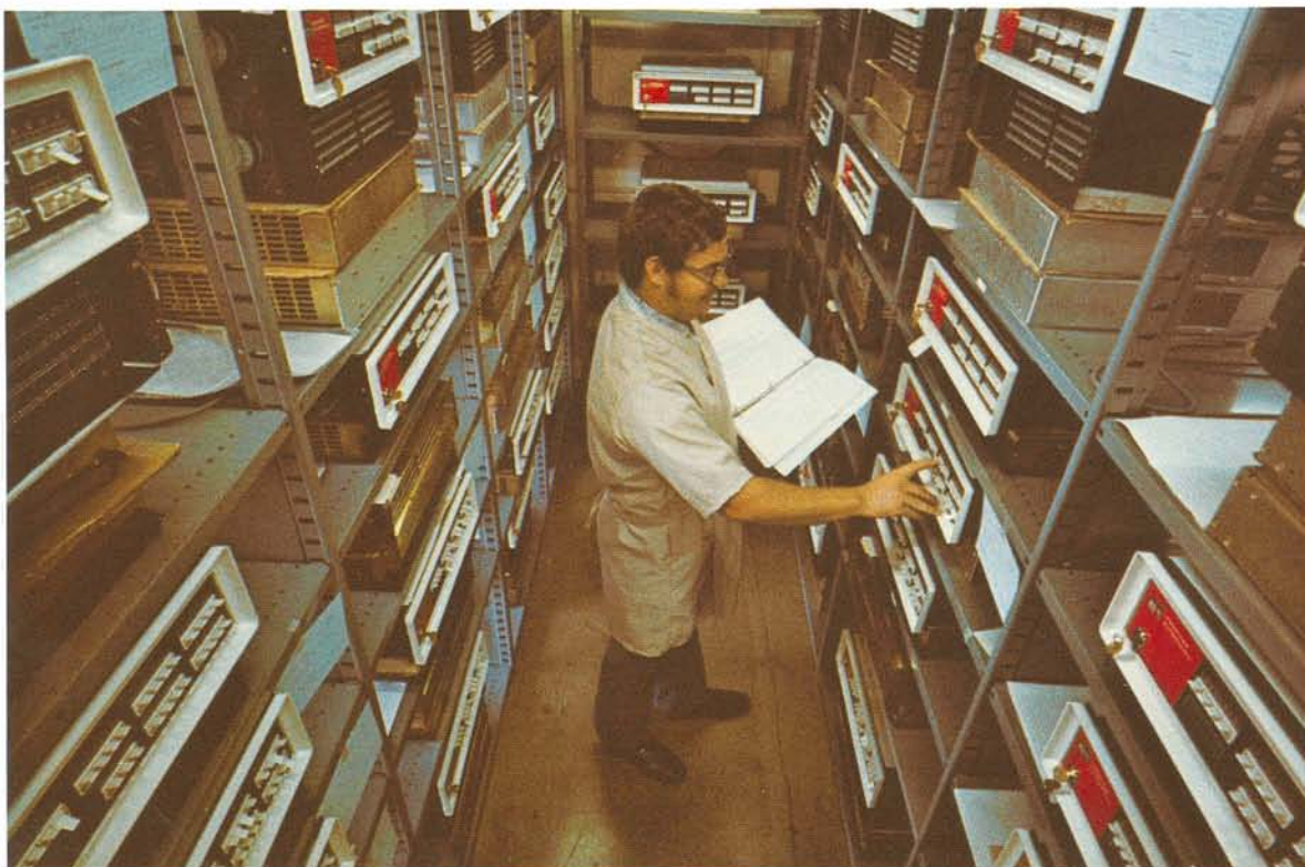
Computers in burn-in undergoing pre-shipment inspection.
